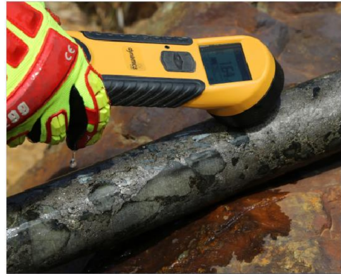
Down-hole magnetic anomaly (pyrrhotite) detected by TruShot and confirmed on surface using a magnetic susceptibility tool
